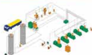
BCS series (Bry-Air Conveying System) 2.2 kw, 4 kw, 7.5 kw to 11 kw with "n" number of station
