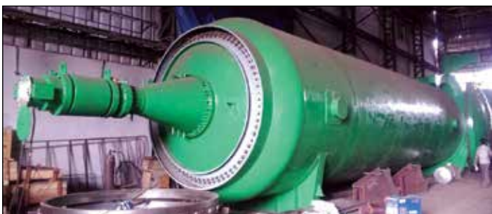
Fig.10: Longest Autoclave designed and Developed (Dia 4m, 15 metre Length) for Advanced System Laboratory (ASL) DRDO, Hyderabad
