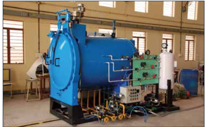
Fig.7 Image of lab scale autoclave developed by CSIR-NAL lead PPP consortium
