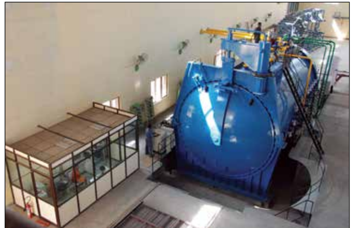
Fig 4. Bird's eye view of the 4.4m x 9 m working space Large Autoclave
