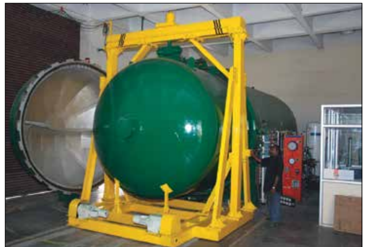
Fig.2: The first Indigenous computer controlled Autoclave with unique dual door technology
