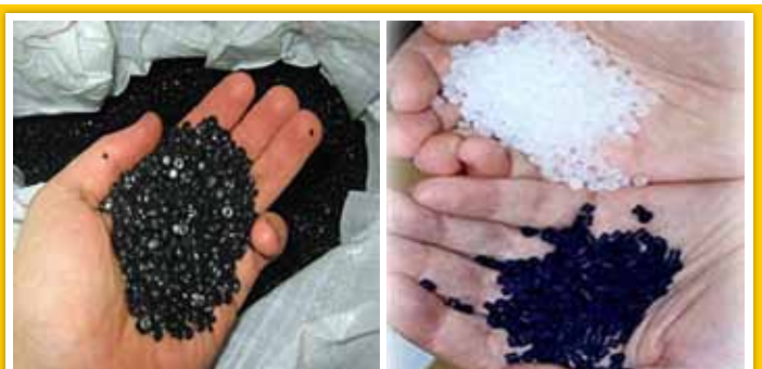
Fig. 1 Pre-Compounded Resin vs Natural Granules to which Black Master Batch is added
