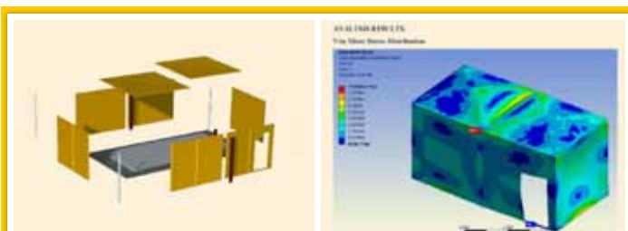
Exploded view Frangible cabin modules
