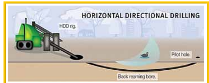
Fig.11 HDD or Trenchless Installation in Graphics
