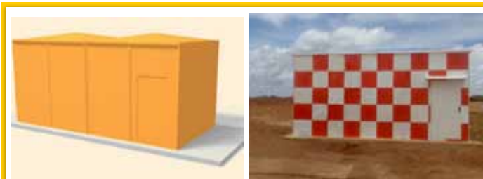
Computer Model of Frangible cabin
